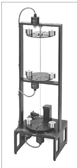
Fig. 1. The ECP Model 205a Torsional Plant (photograph taken from the manufacturer's website http://www.ecpsystems.com )
