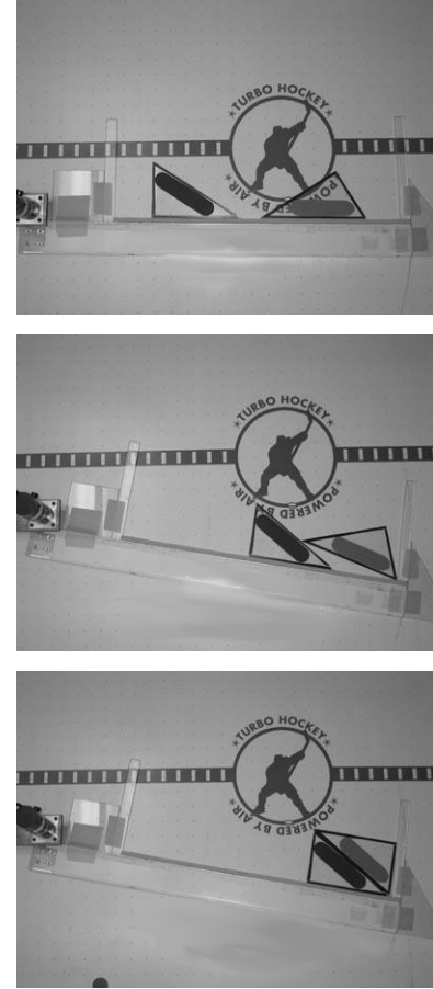
Fig. 15. Three snapshots of the two parts being assembled. Top: parts are in the basin of attraction of the assembled state under the high-priority low-energy throwing map. Middle: a partial assembly. Bottom: the final assembly.
