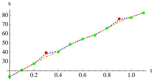
Fig. 6: The dot-dashed orange line represents the mean trajectory of the SSBDA algorithm using a PDAF in the update step. The dotted blue line represents the mean trajectory of the SSBDA algorithm using a Kalman filter in the update step, i.e., does not include any probability of association.
