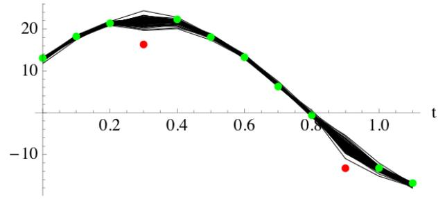
Fig. 4: SSBDA using a PDAF for the nonlinear system. The red points are erroneous measurements, the green points are correct measurements, and the black lines are the stochastic trajectories.
