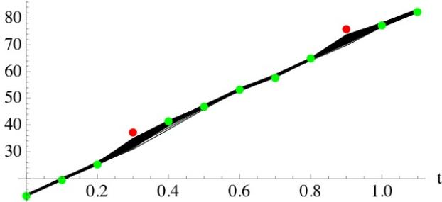
Fig. 2: SSBDA using a PDAF for the linear system. The red points are erroneous measurements, the green points are correct measurements, and the black lines are the stochastic trajectories.
