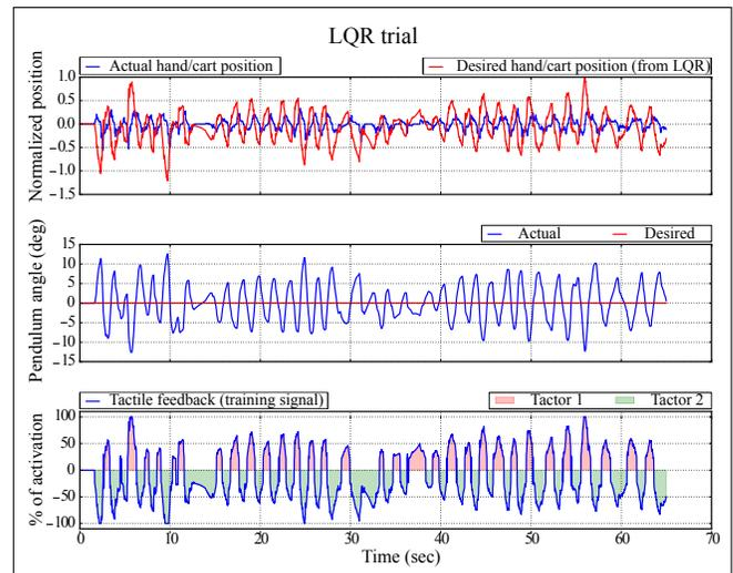
Fig. 4. Typical response of a subject training with both tactile and visual feedback. The percentage of activation is equivalent to the amplitude of vibration.
