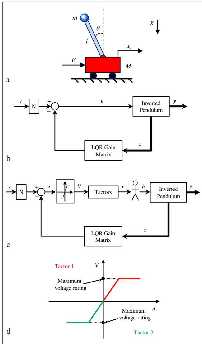
Fig. 2. (a) A schematic of the inverted pendulum/cart system. The rod is considered massless. (b) A typical LQR control loop. (c) Extended LQR loop where the controller is used to “teach” the user how to balance the system. (d) Mapping from  $u$  to  $V$ . All symbols are explained in Table I.
