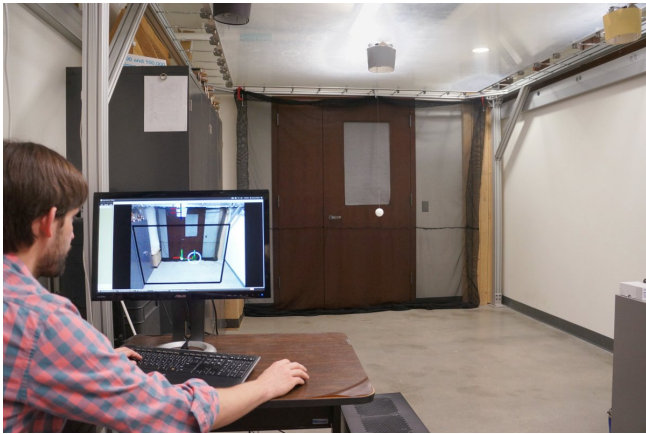
Fig. 3: An image of a user controlling the interactive, receding horizon controlled suspended mass system.
