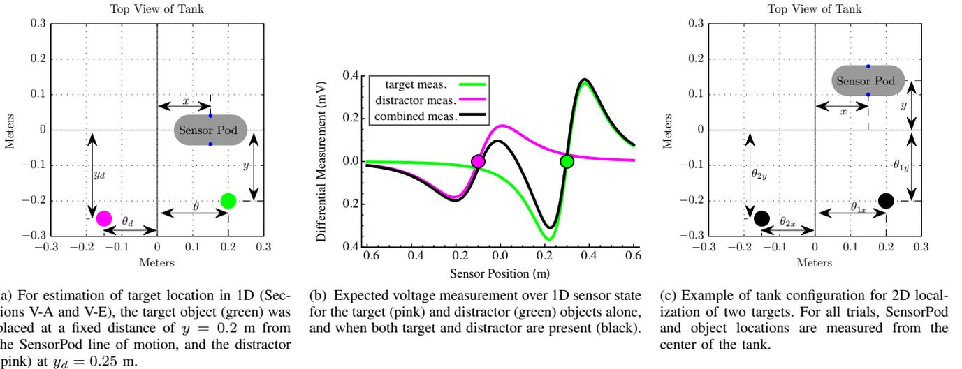
Fig. 7. Targets were placed below the robot’s plane of motion to prevent collisions. The orientation of the robot is held constant. The voltage sensors sample at 100 Hz, with an assumed standard deviation of  $100 \mu V$  for the measurement noise, the experimentally observed noise level of the SensorPod sensors.
