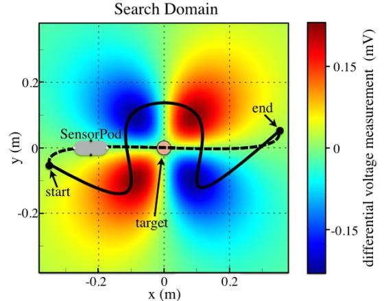
(a) The expected differential voltage measurement (A-B from Fig. 4) is plotted as a function of robot centroid for a target (pink) located at  $X,Y=(0,0)$ . Two possible SensorPod trajectories are plotted in black (solid and dashed). The target is placed below the robot’s plane of motion to prevent collisions.
