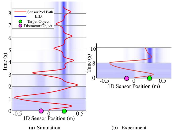
Fig. 8. Examples of closed-loop optimally ergodic search in simulation and experiment. The EID is shown as a density plot in blue, and the search trajectory in red. The belief and trajectory are recalculated every second in simulation and every 8 seconds in experiment.
