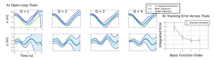
Fig. 5. Here we show reference tracking using open-loop trajectory optimization. The reference trajectory was made sufficiently aggressive to excite the system's internal nonlinearities that cannot be captured completely by the minimal state representation. Respective integrated tracking errors are shown to decrease with an increase in Q. This suggests that the approximate Koopman operator better represents the dynamics of the system with increasing complexity of  $\Psi$ .
