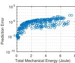
Fig. 2. Simulated trajectories when the approximate Koopman operator was used to propagated the system's configuration. As the complexity  $\Psi$  increases, so does the accuracy in prediction. 100 trials with uniformly random initial conditions were conducted to investgate the relationship between accuracy and total mechanical energy. The prediction error tended to increase with total mechanical energy.
