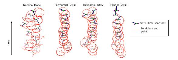
Fig. 4. Each Koopman operator is trained on the residual modeling error of 20 seconds attempted pendulum inversion using the nominal model. As the order of the polynomial basis increases from  $1 \to 2$ , the number of swing up attempts also increases. Notably, a first order Fourier basis captures the necessary features that allow the controller to invert and stabilize the pendulum. Link to multimedia provided: https://vimeo.com/219458009.
